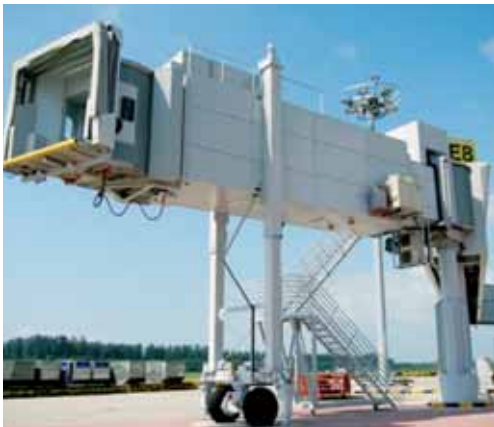
Provision of 3rd arm PBB for A380 (NLA) gate at Singapore Changi Airport Terminal 2
