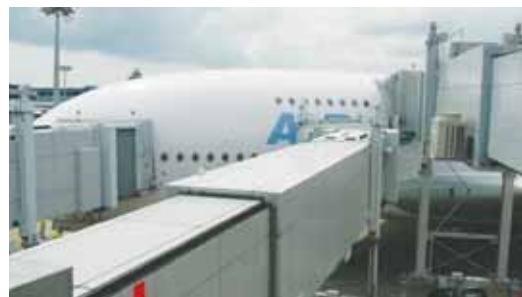
Three arms docking to A380 airbus at the same time.
